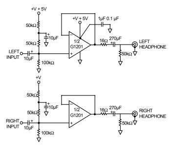
Figure 2. A Single-Supply, Stereo Headphone Driver
